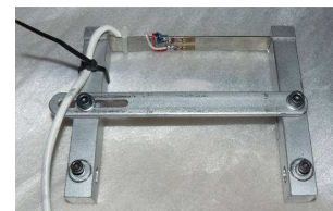
Figure 1 – Stain gauge based deformation device.
