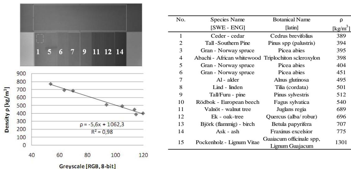
**Figure 1** – Verification of the greyscale density calibration method on a timber specimen (right) using a number of specimens (left) to correlate the density with.
