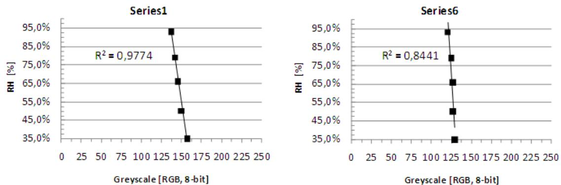
**Figure 2** – Examples of results from the differences in of greyscale due to differences in RH
