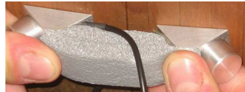
Figure 1 - Crack depth determination
